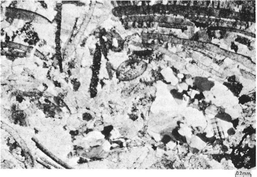
Fig. 2. Middle Cambrian (1c) trilobite biosparite with clasts of microcline gneiss (1.2 mm). Loc. Slemmestad. Crossed nicols.
