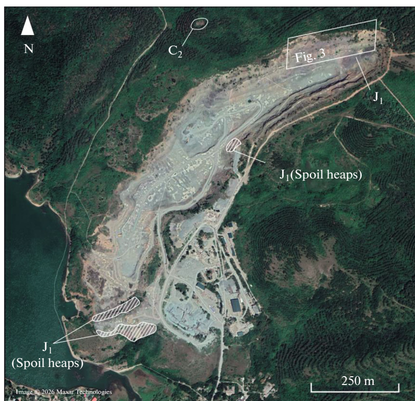
Fig. 2. Location of spoil heaps containing boulders of Lower Jurassic limestone at the Lozovoe Quarry. Satellite imagery from Google Earth (imagery date: 05.07.2019).
